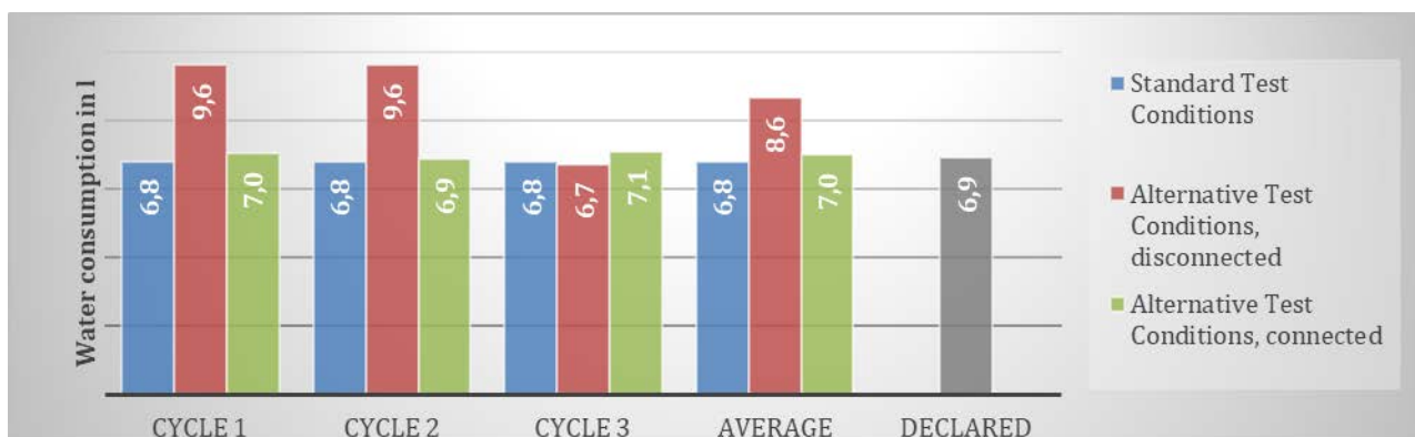
Figure 4-2: Comparison of the water consumption for the three test cycles of Case DISH 2 (regeneration operations excluded)
